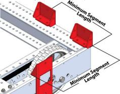
**NOTE:** Screws holding the chassis corner will need to be removed to install brackets on the corner.
